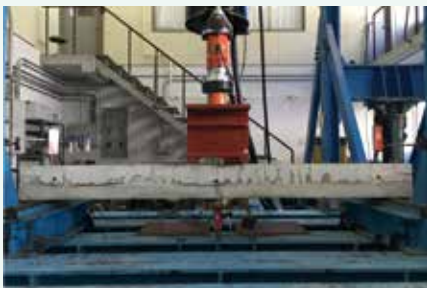
Static loading test
